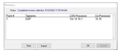
In the example above, the controller was selected prior to initiating the "Get Revision" command. The "Revisions..." dialog box displays the controller's information.
