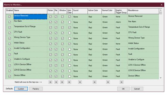
This scrolling list displays the alarms and events related to the device that can be configured to be monitored by S<sup>3</sup>. There are 28 alarms and events that pertain to the status and diagnostics for the IR X9800.
