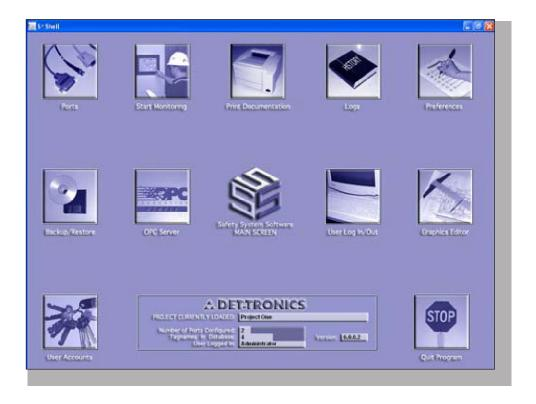
Before any work can be performed, the user must "log in" to the system with a valid password utilizing the "Log In/ Out" button. The options available pre-login are Print Documentation, Logs, and Quit Program.
