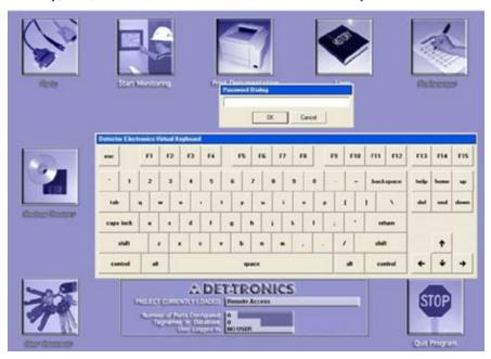
This is primarily to provide user input on systems equipped with a touchscreen as the operator's primary interface.
