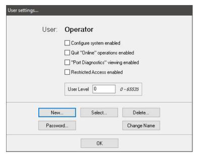
There are four check boxes and one field that are used to configure the user's account.
