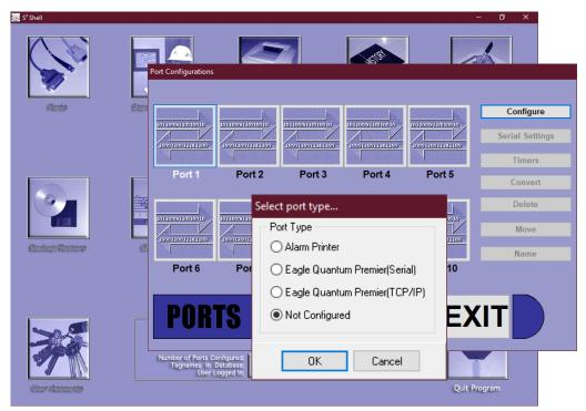
"Not Configured" is the default selection. Simply select the radio button for the type of port to be created and click "OK". This will open the main configuration screen for the selected port type. Clicking "Cancel" will return to the Port Configurations dialog box without any change. Selecting either of the Eagle Quantum options and clicking "OK" will open the LON overview screen as below.
