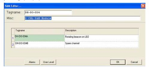
Below, the tagname is a "Misc" text field to enter descriptive information to better identify the location or purpose of the module. Data in this field is optional.
