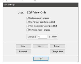
When a user account is created using only the restricted access checkbox, the user can log in and view the configuration and calibration logs, as well as configure and initiate the print-out of system documentation but cannot access any other S³ features.
