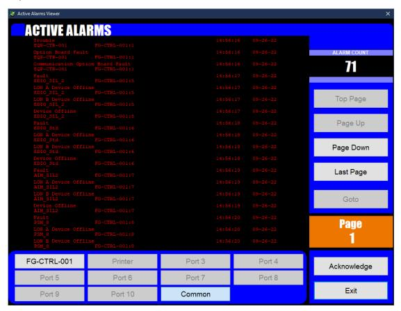
There is a counter at the top right indicating the current number of active alarms. In the lower right, there is a page indicator and buttons for acknowledging alarms or exiting the display.
