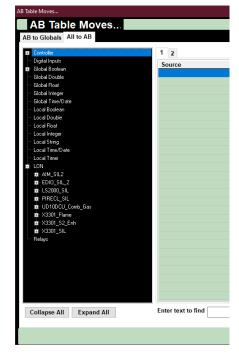
In the example below, a field device on the LON, an EDIO Module with the tagname "EDIO\_SIL\_2" has been selected and "opened" to display its subordinate data. Any of the displayed items can be selected and configured for "movement" to the AB system utilizing the "drag and drop" method.
