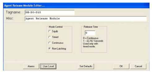
The release circuits are compatible with a variety of solenoid or initiator (squib) based suppression systems. The release circuit is supervised for open circuit conditions. If a trouble condition occurs (open circuit or solenoid supply voltage less than 19 volts), it will be indicated at the controller.
