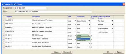
Being a multi-channel device there are multiple tagnames. At the top of the dialog box there is a device tagname that refers to the DCIO or EDIO module and is used with its global status and diagnostic events. Below this are channel tagnames for the status and diagnostics relating to the eight individual channels.
